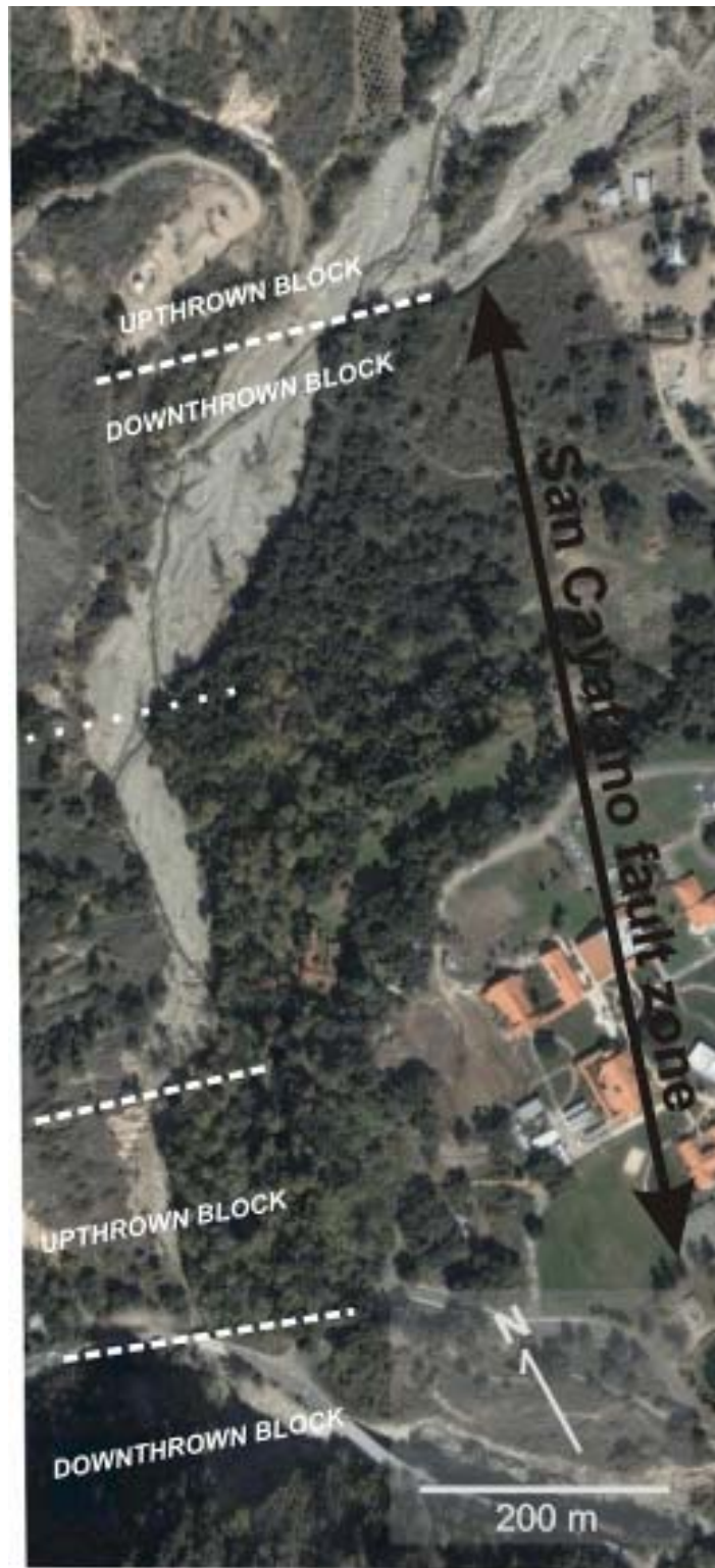
Figure 2-17. Santa Paula Creek crossing of the San Cayetano fault. Dashed lines show mapped strands; the dotted line is unmapped but is strongly suggested by the pattern of bedrock outcrops. Over the course of about 1 km, the transported sediment load of the channel is apparently reduced by a substantial fraction, as indicated by the width of the active meander/braid belt upstream of each valley narrowing. Assessing tectonic-related changes in transport through this reach is confounded by the correspondence of the southern-most fault crossing with the Highway 150 bridge.
